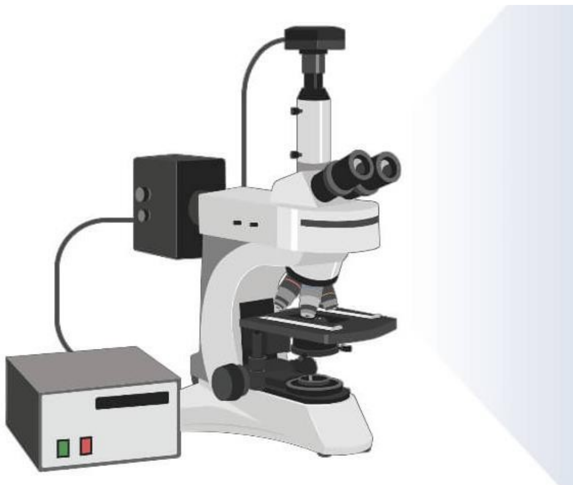
Fig. 2.3: Structure of Fluorescence Microscope
