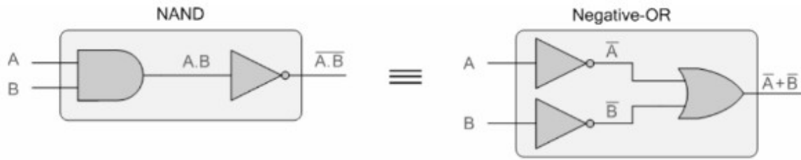
Figure 1.5 Demorgan's first theorem
