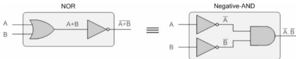
Figure 1.6 Demorgan's second theorem
